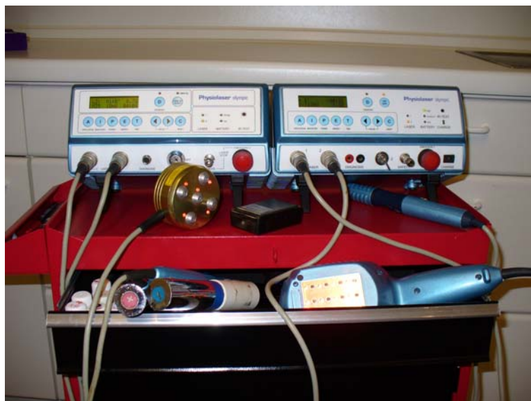
Figure 2a, left: Two Physiolaser Olympic low level impulse lasers units a each with a single probe and a cluster probe). Both Physiolasers are connected with one 90 watt single probe for acupoint stimulation and topical therapy (A). The left unit also has a 5 x 30 watt impulse laser shower (B) and the left unit also has a 12x 10 watt impulse laser shower (C) for topical therapy; Figure 2b, right: Laser Pen a 40 W/904nm for acupoint stimulation in charging station.
